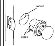
outside knob assembly with two 10-24 x 1-1/4" machine screws.
