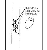
diameter pilot holes for #8 x 3/4"
