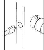
Align the strike and trace an outline onto the door frame using the mounting screw marks for locadates both size backsets.
