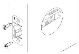
⚠ Make sure the slant of the latch bolt faces in the direction that the door closes.
