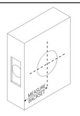
⚠ If backset of door measured 2-3/4" (70mm), adjust latch shown by prograsping the spring pin and moving it to the 2-3/4" slot.
