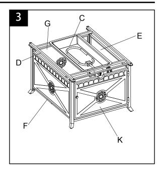
4. Attach the 4 - Bolt(8\*50mm) (L) to the corners of the Table Top (B). Then align the Bolts with the holes in the Burner Bracket and assembled panels and insert the Bolts through the holes. Secure the Table Top to the Burner Bracket and assembled panels with 4 - Washer/Spring Washer/Nuts (L).
