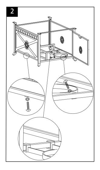
Put the Burner Bracket(D) on the unit.
