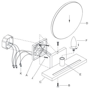
4.GENTLY PULL THE ELECTRICAL CORD FROM JUNCTION BOX, THEN PULL THE ELECTRICAL CORD FROM BACK PLATE THROUGH THE EXIT HOLE OF THE MOUNTING PLATE PLATE THROUGH THE EXIT HOLE OF THE MOUNTING PLATE PLATE
