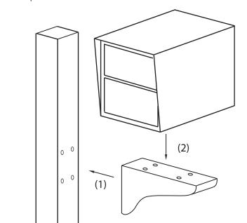
For double configurations (one mailbox on each side of the post), assemble both support arms (5512) as shown above. Double configurations can be used for Coronado, Bellevue or Oasis Jr. Mailboxes.
