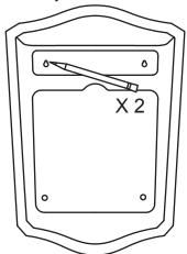
For brick or other masonry wall, insert a plastic anchor (included) into each hole. Tap in gently if necessary. This step is not required if mounting on a wood wall.
