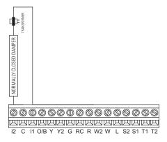
Note: The I1/I2 output is a dry contact closure. The humidifier wiring diagram assumes the control is powering a solenoid valve. The dehumidifier wiring diagram is for a normally open dry contact input. The ventilation diagram assumes the control is for a normally closed damper. Refer to the individual humidifier, dehumidifier or ventilation installation instructions for product specific wiring details.
