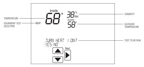
While the equipment test is active the corresponding test information will be shown.
