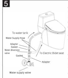
①Close the water supply stop. Disconnect the water supply hose of the toilet and the supply stop;
