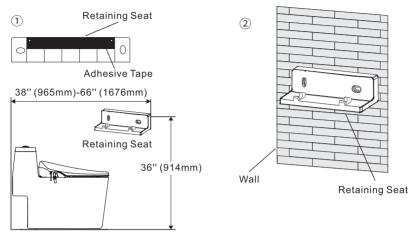
Select a smooth and even surface to ensure the control holder remains seated.
