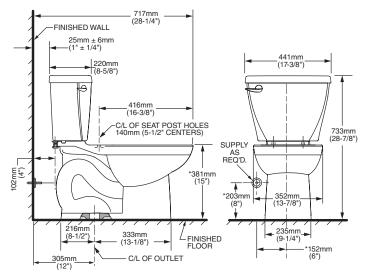
NOTES: THIS TOILET IS DESIGNED TO ROUGH-IN AT A MINIMUM DIMENSION OF 305MM (12") FROM FINISHED WALL TO C/L OF OUTLET. SUPPLY NOT INCLUDED WITH FIXTURE AND MUST BE ORDERED SEPARATELY. \* DIMENSION SHOWN FOR LOCATION OF SUPPLY IS SUGGESTED.
