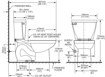
THIS TOILET IS DESIGNED TO ROUGH-IN AT A MINIMUM DIMENSION OF 254MM (10") FROM FINISHED WALL TO C/L OF OUTLET. SUPPLY NOT INCLUDED WITH FIXTURE AND MUST BE ORDERED SEPARATELY. \* DIMENSION SHOWN FOR LOCATION OF SUPPLY IS SUGGESTED.
