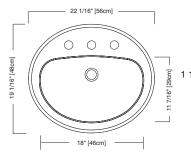
13SR.182143.073 Standard drilling: 3 hole 1 1/2" dia., 8" centers
