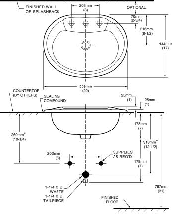
NOTES: \* DIMENSIONS SHOWN FOR LOCATION OF SUPPLIES AND "P" TRAP ARE FOR COUNTERTOP CUTOUT AND INSTALLATION INSTRUCTIONS USE TEMPLATE SUPPLIED WITH SINK. FITTINGS NOT INCLUDED WITH FIXTURE AND MUST BE ORDERED
