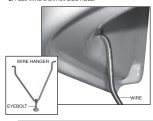
3. Place WIRE end in right SIDE HOLE near DRAIN.
