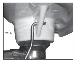
NOTE: If not enough tension, remove WIRE and spread ends approx. 1" additional and re-attach.
