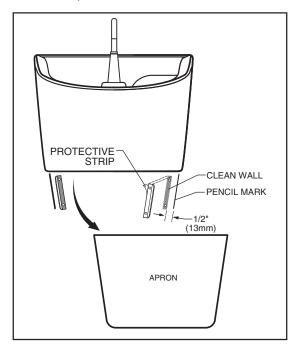
5. Position APRON under SINK and against finished wall alinging EYEBOLT with hole in APRON.
