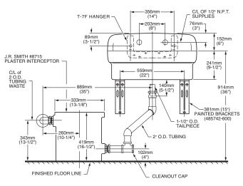
NOTES: SHOWN WITH J.R. SMITH NO. 8715 PLASTER INTERCEPTOR. FITTINGS NOT INCLUDED AND MUST BE ORDERED SEPARATELY. 15" PAINTED SUPPORT BRACKETS 485742-600 AVAILABLE AND MUST BE ORDERED SEPARATELY. PROVIDE SUITABLE REINFORCEMENT FOR ALL WALL SUPPORTS.
