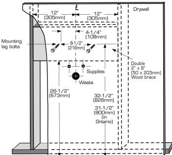
Finished floor Figure 1 Concealed arm carrier holes Basin anchor holes Figure 2 Slots for basin lag bolts Bend flexible supply tubes Semi-pedestal/shroud anchor holes Figure 3 3-3/4" 7-3/4" (63 mm) 7-1/2 (197 mm) (191mm) 9-3/4" (248 mm) Supplies \*34" (864 mm) Waste 10" (254 mm) 33" (838 mm)
