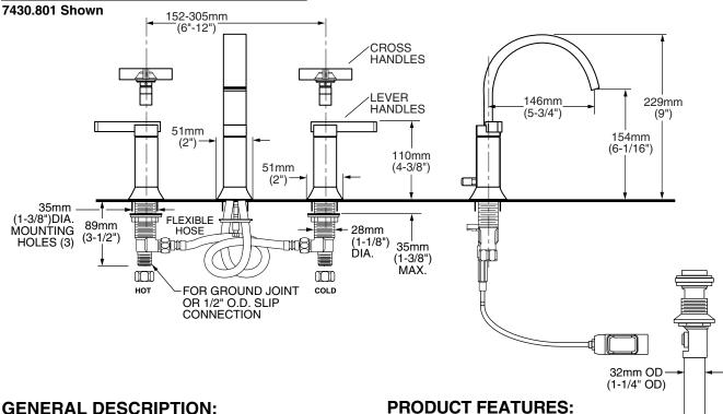
Cast brass valve bodies with flexible hose connections for 6" to 12" (152mm to 305mm) installations. 1/4 turn washerless ceramic disc valve cartridges. Brass spout. Choice of metal lever or metal cross handles. One-half inch male inlet shanks with brass coupling nuts. 20 inch (500mm) long flexible stainless steel drain cable is pre-assembled to spout. Metal Speed Connect® drain body with 1-1/4 inch (32mm) tail piece. 1.5 gpm/5.7L/min. maximum flow rate.
