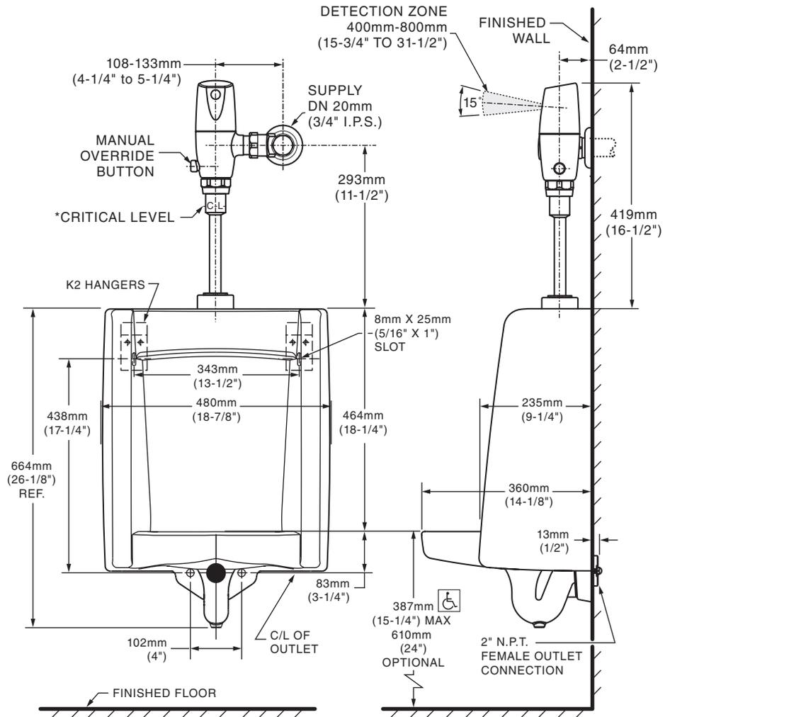
\*Note: The Critical Line (-C-L-) on Vacuum Breaker must typically be a minimum of 6" (152mm) above fixture. Consult Codes for details.
