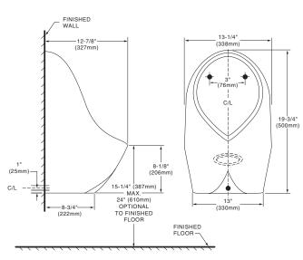
**NOTES:** PROVIDE SUITABLE REINFORCEMENT FOR ALL WALL SUPPORTS.
