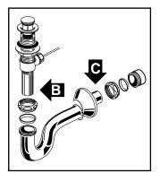
Secure lavatory to wall as shown in 5 or 5a. Install washers and hand tighten nuts or lag bolts. Level and square the unit. Connect hot and cold supply lines to the shut-off valves. Tighten trap joints for watertight assembly.
