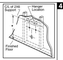
Place lavatory and pedestal into installed position. Level and square the lavatory and pedestal assembly. Use one or more bumper cushions (supplied) to level and cushion lavatory slab to pedestal.
