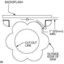
Drill a clearance hole inside the perimeter line of the template.
