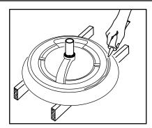
After checking fit and alignment, turn sink upside down and apply a generous portion of sealant around the under side of the rim near the edge.
