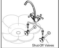
Connect supply line to faucet (finger tight) and carefully bend tubes to engage with the supply shut-off valves. Tighten connections at faucet and shut-off valves for secure seal.
