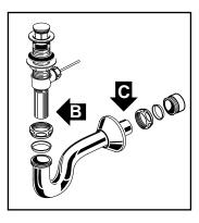
Connect trap to drain assembly hand tight to check alignment. It may be necessary to cut off part of the tailpiece (area "B") or part of the horizontal leg of the trap (area "C"). Secure joints for watertight assembly.
