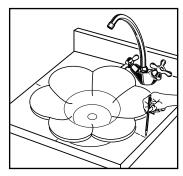
Before applying the sealant, place the sink temporarily into the cutout. Check for alignment and clearance. Then mark the sink and countertop in several places as a guide for the installation location.
