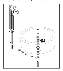
Before applying the sealant, place the vessel temporarily into the cut-out. Check for alignment and clearance. Then mark the vessel *and* countertop in several places as a guide for the installation location.
