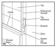
Draw a line 6-5/8" (159mm) from the sub-floor on to the studs at each side of the opening. Using this line and a level, mark the remaining studs. (See Figs. A & B.) This will be the installed height of the shower base. Mix the low-shrink bedding material (grout, mortar, plaster, etc.). Concrete is not recommended. Apply enough bedding material to support the entire bottom of the shower base. The bedding material must not be used under the apron (front edge).
