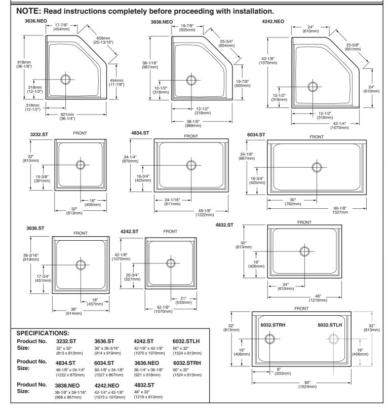
Insure the floor and stud walls are square and plumb. Provide a 5" x 5" (127mm x 127mm) opening in the floor for the drain (see Figs. A & B). The drain plug accom-modates a 2" (51mm) **PVC** waste pipe. The waste pipe should extend above the surface of the sub-floor, refer to chart on page 2 for the required dimensions. See product drawings on this page for the specified drain locations.
