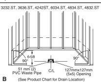
Note: Variations in levelness of the subfloor may require adjustment of waste pipe height.
