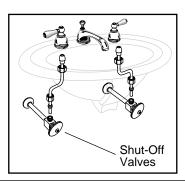
5 After checking fit and alignment, turn sink upside down and apply a generous portion of sealant around the underside of the rim near the edge. Carefully lower sink in place, align with marks made earlier, and press downfirmly. Allow sealant to set before connecting supplies and drain.
