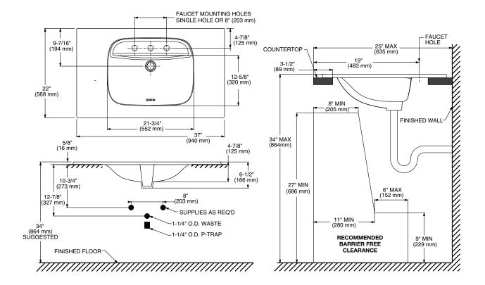
MEETS THE AMERICANS WITH DISABILITIES ACT GUIDELINES AND ICC ANSI A117.1 ACCESSIBLE AND USABLE BUILDINGS AND FACILITIES - CHECK LOCAL CODES. Install lavatory 864 mm (34") from finished floor. Lavatory installed 89 mm (3-1/2") minimum from front edge of countertop provides 686mm (27") knee clearance area.
