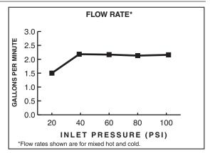
2.2gpm/8.3L/min. FLOW RATE
