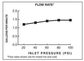
1.5gpm/5.7 L/min. FLOW RATE
