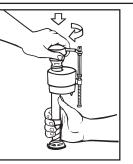
Replace TOP by engaging lugs and rotating 1/8 turn clockwise. MAKE CERTAIN TIP IS TURNED TO THE LOCKED POSITION. VALVE MAY NOT TURN ON IF TOP IS NOT FULLY TURNED TO THE LOCKED POSITION. TROUBLESHOOTING
