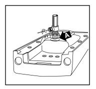
Return the fitted lavatory to the installed position. Connect trap to drain assembly hand tight to check alignment. It may be necessary to cut off part of the tailpiece (area "B") or part of the horizontal leg of the trap (area "C").
