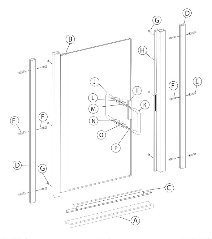
The 1/4" frameless door is completely reversible and may be installed hinge-right or hinge-left. Refer to the illustration to determine the best hinge position for your installation.
