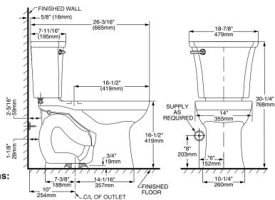
THIS TOILET IS DESIGNED TO ROUGH-IN AT A MINIMUM DIMENSION OF 254MM (10") FROM FINISHED WALL TO C/L OF OUTLET.
