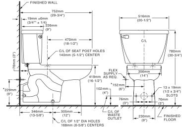
WASTE OUTLET SEAL RING MUST BE NEOPRENE OR GRAPHITE-FELT (WAX RING NOT RECOMMENDED). SUPPLY NOT INCLUDED WITH FIXTURE AND MUST BE ORDERED
