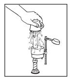
While holding a container over the uncapped VALVE to prevent splashing, turn water supply on and off a few times. Leave water supply off.
