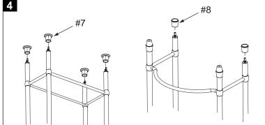
Thread one decorative foot (Item #7) onto the end of each rod until the leading end of the rod is recessed with the foot to a depth of 1/4". **Set the unit upright** and thread one leveling trumpet (Item #8) on the top of the rear legs.
