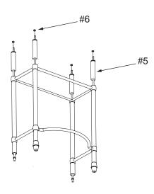
Place a bottom leg tube (Item #5) over each threaded rod such that the closed end of each is nearer to you. Thread one hex nut from the kit (Item #6) onto each rod. Lay the unit down and tighten each of the four legs firmly. Maintain the 5/8" of exposed thread at the top end of the rear legs. Once again, set the unit upside down.
