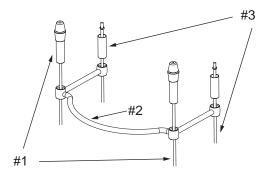
Run the two front leg sub-assemblies (Item #1) through the two front holes of the towel bar (Item #2). Do the same with the two rear leg assemblies (Item #3). Adjust the hex nut at the end of each rear leg such that 5/8" of thread is exposed. **Turn the unit upside down.**
