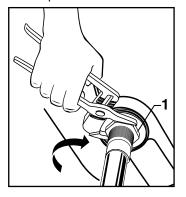
and FLANGE (4) onto drain tighten FLANGE (4) firmly.
