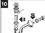
Connect trap to drain assembly hand tight to check alignment. It may be necessary to cut off part of the tailpiece (area "B") or part of the horizontal leg of the trap (area "C"). Secure joints for watertight assembly.
