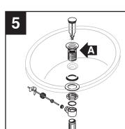
Mount the drain assembly (not included) on the sink, following faucet manufacturer's instructions. Be certain to apply a bead of sealing putty on the underside of the drain (Part "A") in order to ensure a watertight seal between the sink and drain. Remove excess putty after installing drain on sink.
