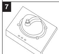
Center bowl over cutout and tighten screws (see step 4) to secure bowl to countertop. Remove excess sealant from inside lip.
