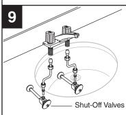
Connect supply line to faucet (finger tight) and carefully bend tubes to engage with the supply shut-off valves. Tighten connections at faucet and shut-off valves for water tight seal.
