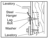
**IMPORTANT:** Final assembly of nut and washer or lag bolt method shown for reference only.
