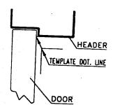
3. Follow template instructions for hole size. Use the illustrations below to determine proper armature mounting hole preparation.
