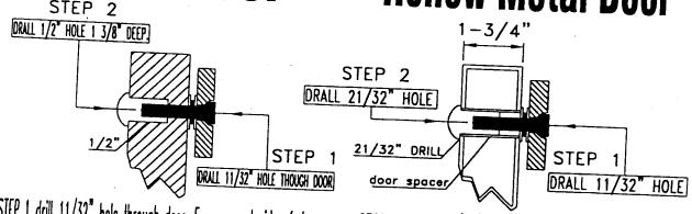
STEP 1 drill 11/32" hole through door. From sexnut side of door STEP 2 drill 1/2" dia. hole 1 3/8" deep. Mount armature to door with hardware provided.
