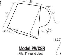
Backdraft damper Galvanized steel construction
