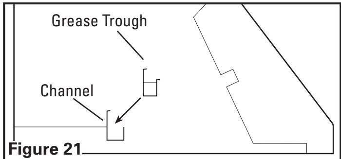
3. Install the baffle filters along with any spacer bars that are required by inserting the top of the filter into the top channel of the hood, then slide the bottom of the filter into the bottom channel. The filters have a top and a bottom. The bottom of the filter will have small drain holes. These holes must be facing down towards the grease trough to be effective. In models with spacers, it is easiest to install the spacer(s) first and the grease filters last (Figure 22).
