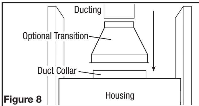
**NOTE:** To transition to round ducting, Air King recommends using model OA10H 4½" x 18" to 10" round transition (not included). When using model OA10H, the existing duct collar must be removed.
