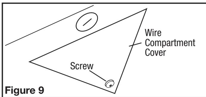
2. Pull the loose black, white and green wires out from the wire compartment (additional wires will be present). Install an approved electrical connector (not included) to the wire compartment cover. Run a black (hot), white (neutral), and a green or bare ground wire from the supply. Connect all wires from the supply to their corresponding wires within the wire compartment (**Figure 10**). Use approved methods for all connections.
