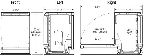
\*Height only adjustable to 35%4" max. when installed in 35%4" max. standard cabinetry cutout. (Dimensions do NOT include insulation – insulation blanket may be compressed during installation.)
