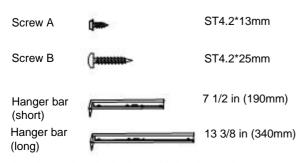
Note: Hanger bar (short) only can slide into channel  ${\sf A}.$
